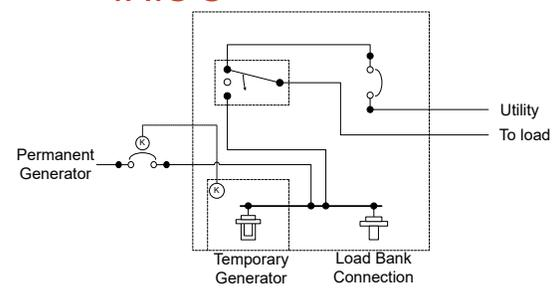
Service entrance rated ATS with dual purpose bank and temporary generator connections
