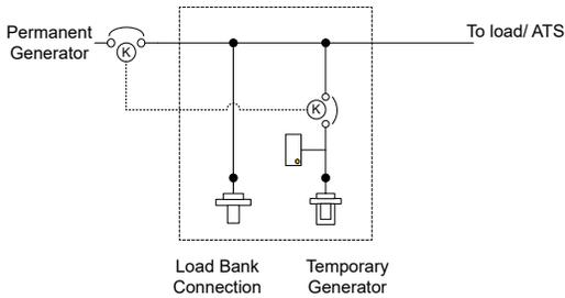
Dual purpose single breaker docking station with male and female camlocks to connect a load bank and temporary power source.
