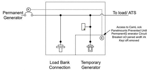
Dual Purpose Docking Station with male and female camlocks to connect a load bank and temporary power source
