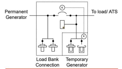
Dual purpose single breaker docking station with male and female camlocks to connect a load bank and temporary power source.
