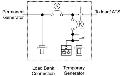
Dual purpose dual breaker with male & female camlocks to connect a load bank or temporary power source. Includes main breaker for the temporary load and permanent line connections.
