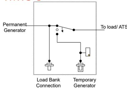
Dual Purpose Manual Transfer Switch to allow the connection of a load bank and temporary power source in compliance with NEC 700.3F
