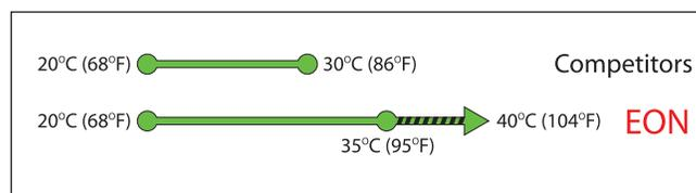
**NOTE:** To satisfy UL 924 and CSA C22.2 No. 141-15 requirements for a 35°C rating, UL testing was performed in a 40°C ambient environment, with units tested under full load and at low line input voltage.
