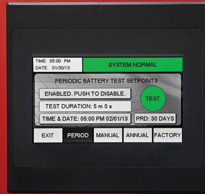
The color touchscreen display on the **Intellistat TS** provides all electrical parameters, inverter status, programmable inverter and battery testing, and data-logging. Optional **Intellistat TS** communications allow for remote monitoring and reporting via **BACnet/IP** or **BACnet MS/TP**, **Ethernet TCP/IP**, **MODBUS TCP**, or **MODBUS RS485**. For more details, see the **Network Communications** description on Page 7.
