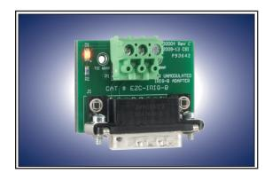
The Cyber Sciences' EZ Connector for IRIG-B (EZC-IRIG-B) or DCF77 (EZC-DCF77) is a wiring adapter for the CyTime™ Sequence of Events Recorder (SER) to facilitate wiring of its precision time-sync input signal. The adapter fits the "Options" port (DB15 connector) of the SER and facilitates wiring of IRIG-B or DCF77 signals via a screw-type terminal, suitable for power equipment wiring. (Model EZC-IRIG-B is shown at left.)
