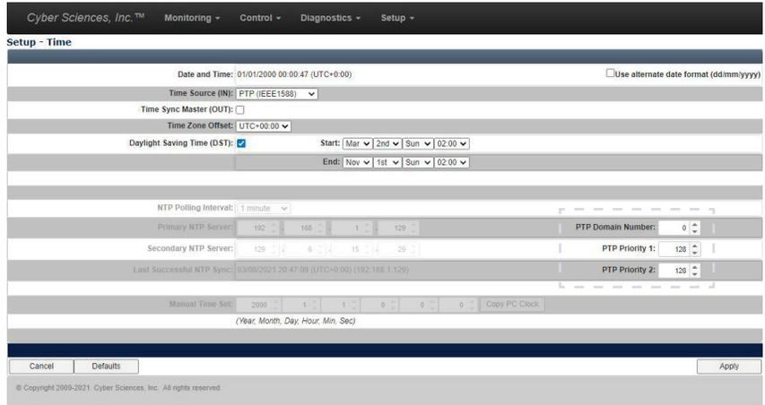
Figure 5-5. Time setup web page (with PTP time source setting shown)
