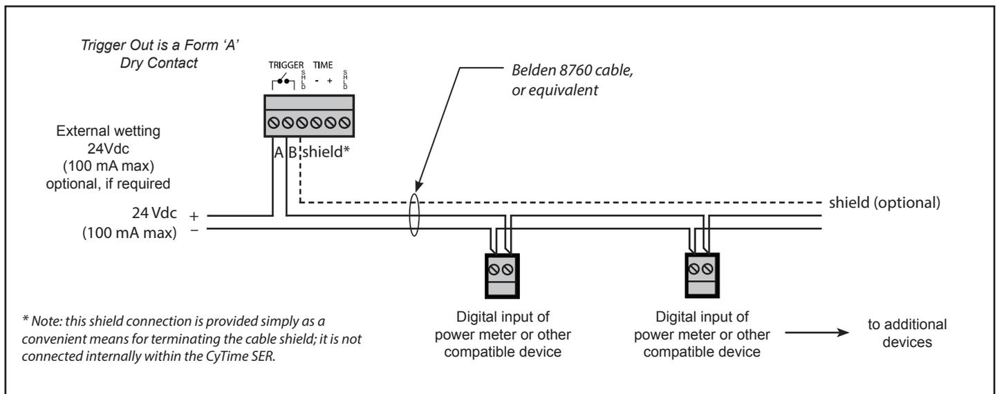
Figure 3-9. Trigger output connection to multiple devices
