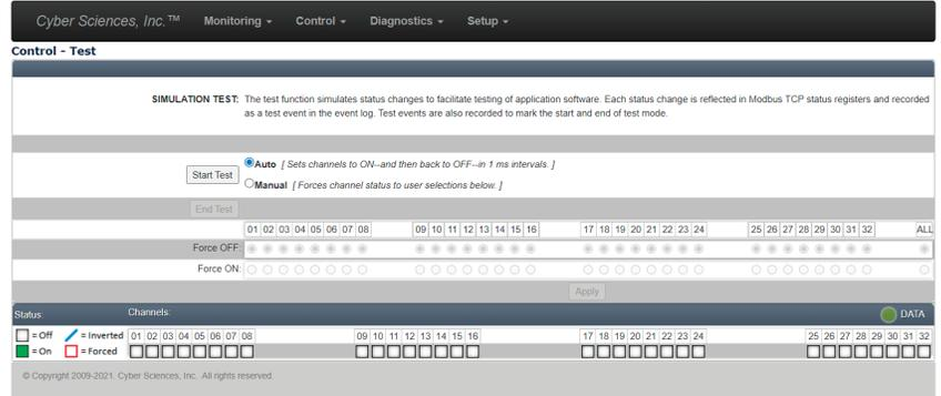
Figure 6-5. Control: Simulation test page (Manual mode shown)
