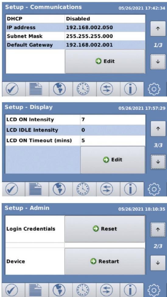
To change communications settings from the SER front panel, select the GEAR icon (⚙️) and press the EDIT button (page 1/3):
