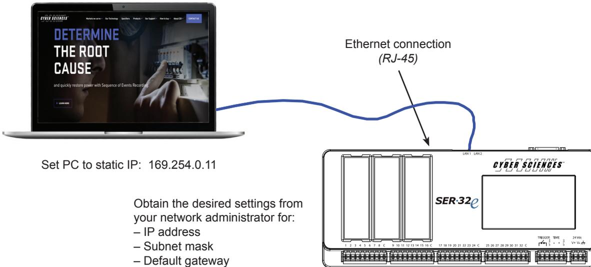
The SER has two (2) Ethernet ports (LAN1 / LAN2). Either port can be used, but only one can be connected at a time. If two ports are connected, only LAN 1 will be active.
