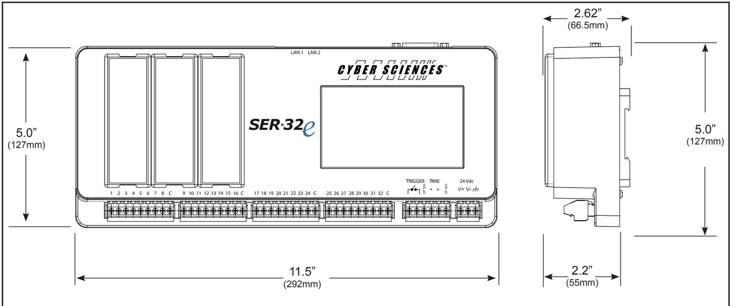
Figure 2-1. Front and side views, with dimensions—SER-32e
