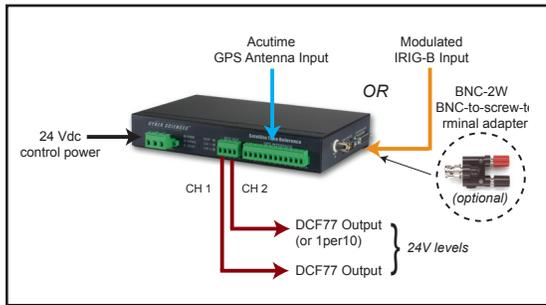
Figure 1-4. STR-100 Inputs/Outputs
