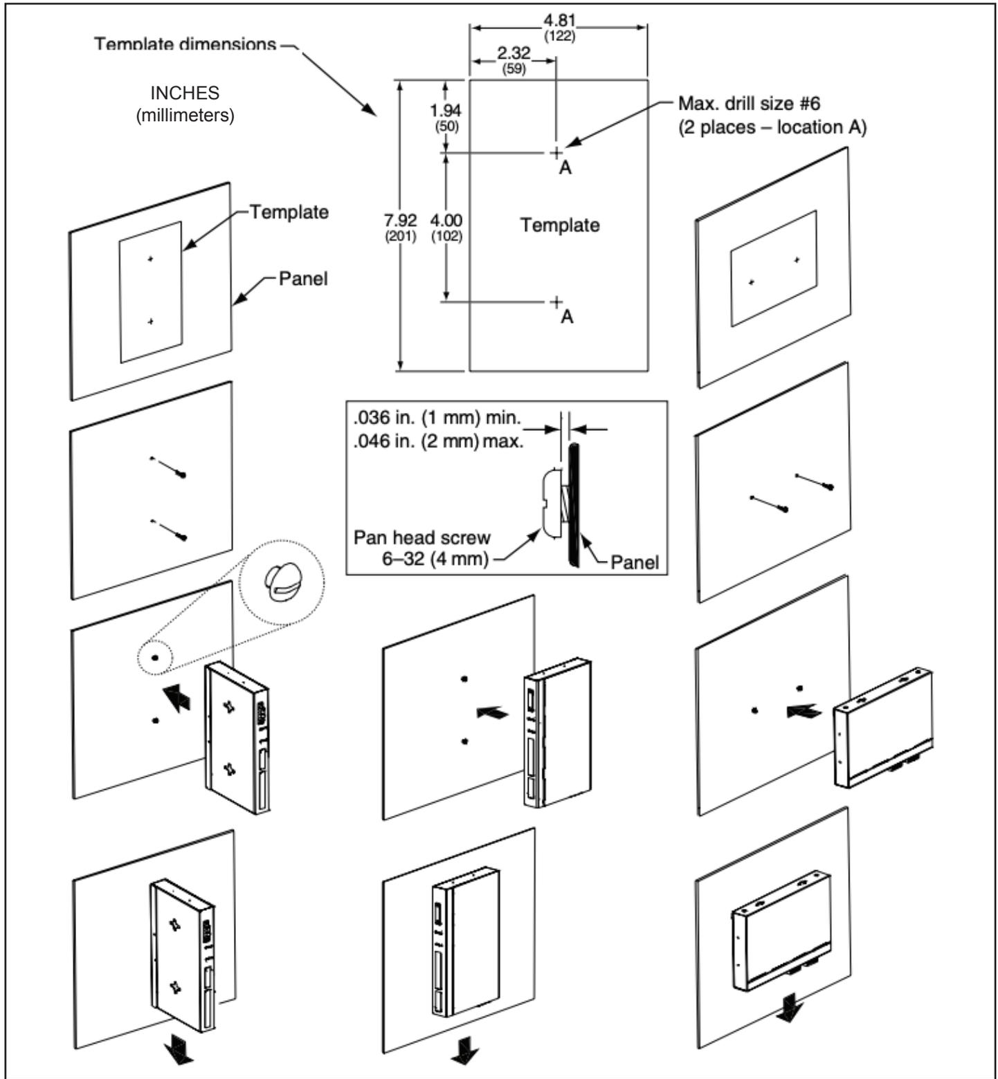
Figure 2-4. Wall / panel mounting of STR-100
