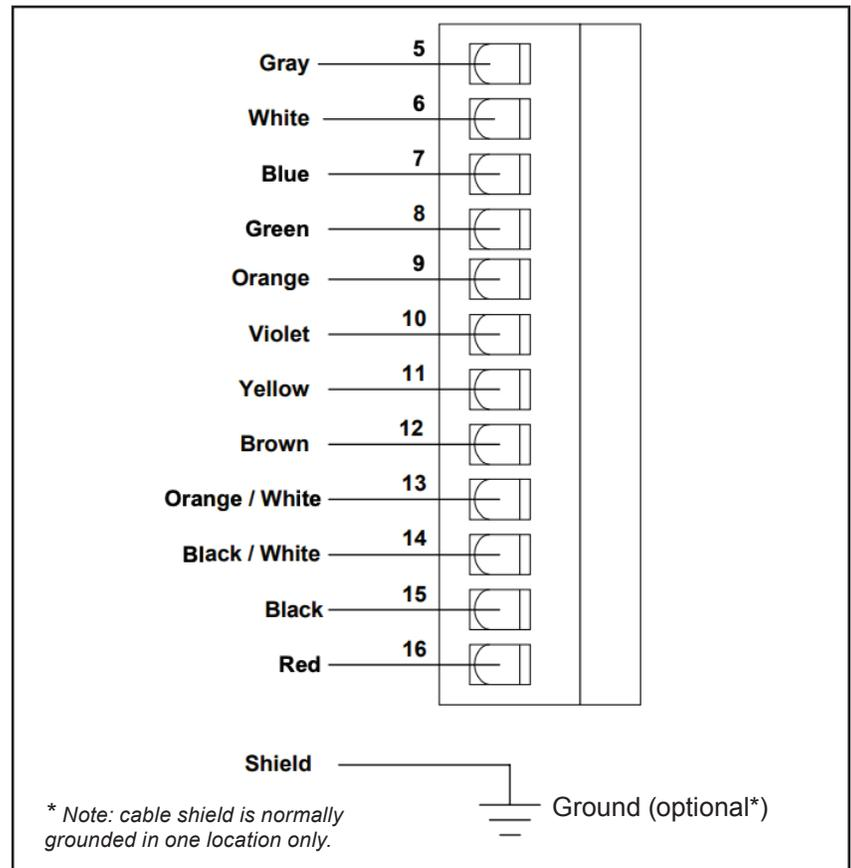
Figure 3-5. Acutime GPS antenna interface connections
