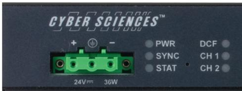
Fig. 5-1. Indicator LEDs (STR front-left)
