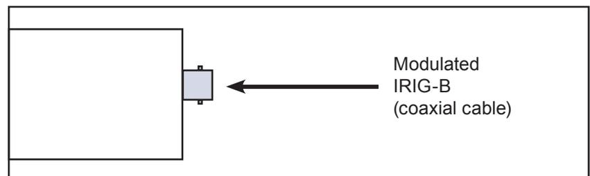
Figure 3-6. IRIG-B input via side BNC connector
