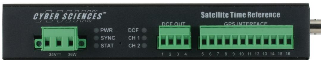
Figure 1-2. STR-100 front view (with connectors removed)
