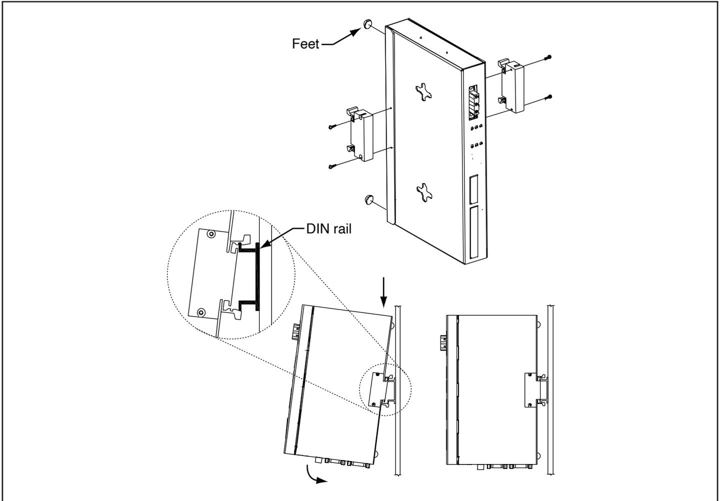
Figure 2-2. STR-100 mounting on standard DIN rail
