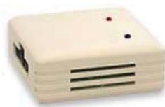
Temperature and Temperature/Humidity sensors are available as options on the NetMinder CS141L. Both of these sensors measure either the ambient temperature and/or humidity, and display the results on a network computer. If the temperature or humidity exceeds the predefined, programmable thresholds, the CS141L will send an e-mail, SNMP trap, or RCCMD command for shutting down servers. This keeps personnel informed and critical equipment protected.
