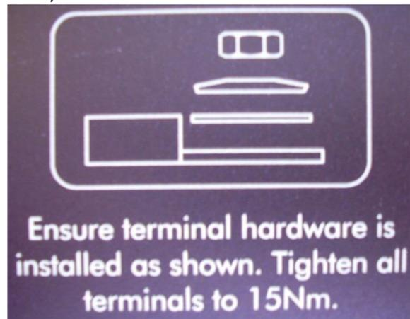
Figure 13: Power Terminal Hardware Stackup
