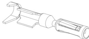
Figure 15: Harness Plug Socket Contact Illustration
