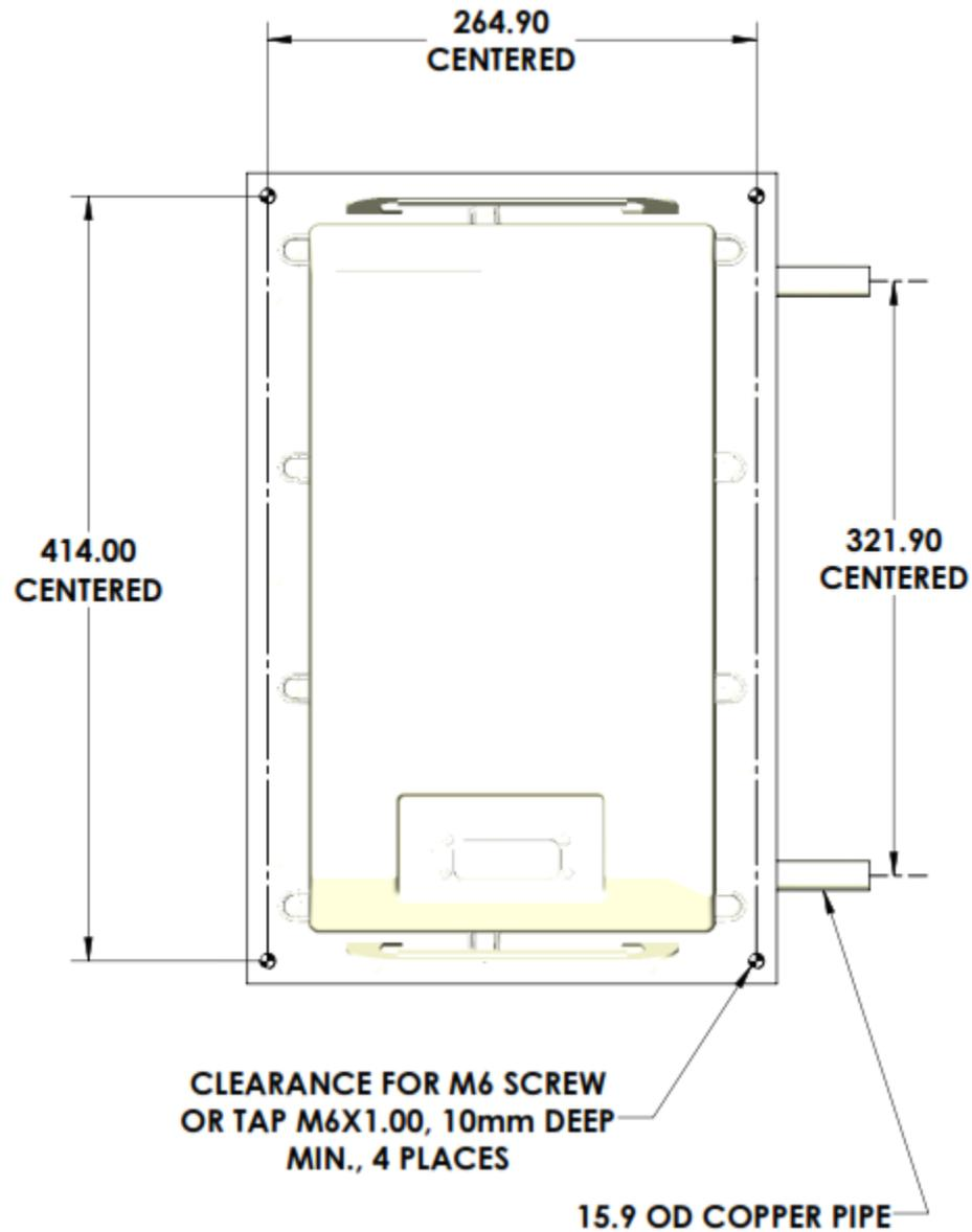
Figure 21: Mechanical Mounting Diagram, Models OZip-R\*\*\*\*L\*\*\*\*
