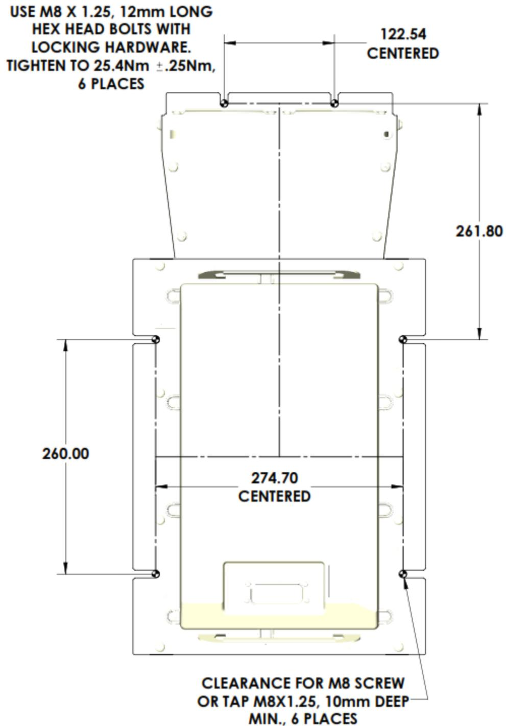
Figure 19: Mechanical Mounting Diagram, Models OZip-R\*\*\*\*F\*\*\*\*
