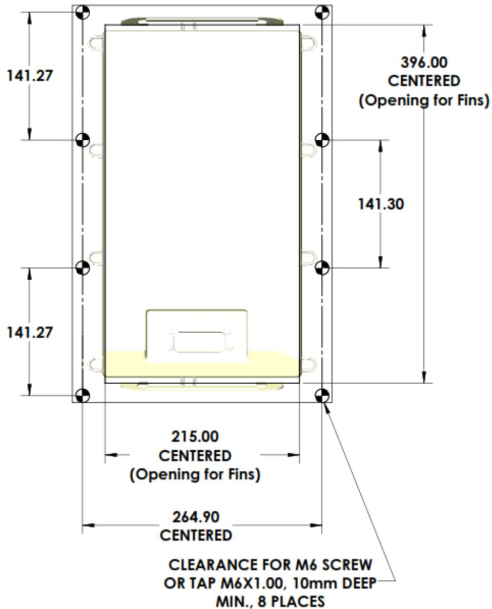
Figure 18: Mechanical Mounting Diagram, Models OZip-R\*\*\*\*E\*\*\*\*
