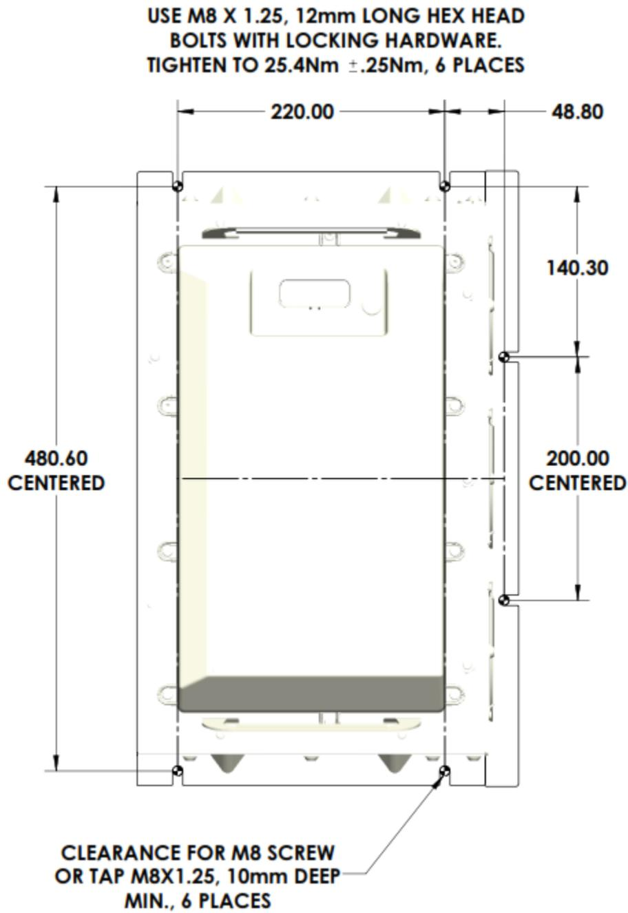
Figure 20: Mechanical Mounting Diagram, Models OZip-R\*\*\*\*H\*\*\*\*
